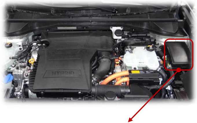
Engine room fuse box
